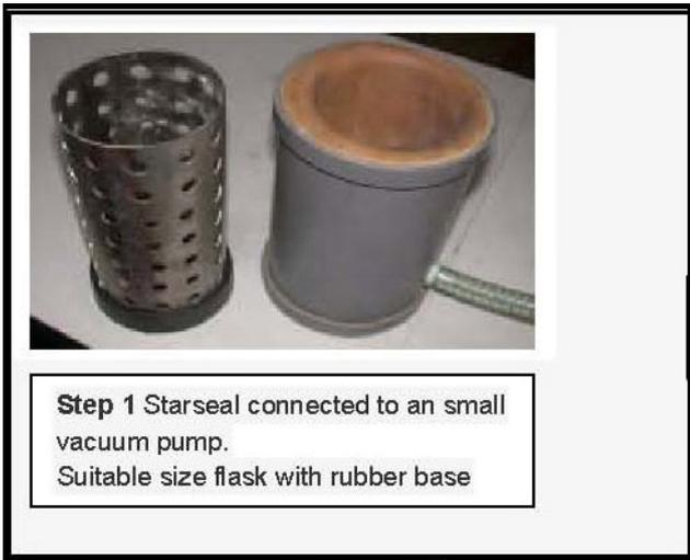
If the method used to **seal the holes** in the flasks while investment in being poured, is not suitable, more **time** will be required, and what is more important:
